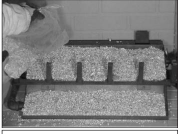
Figure 4 Placing Vermiculite
